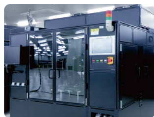
Camera module fully automatic tester
