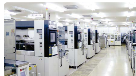
Backside polishing, laser grooving, Wafer dicing.
