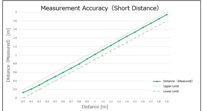
Short Distance Measurement Accuracy (Gain: +14dB)
