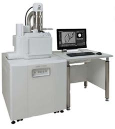
The decapsulated sample is observed with high accuracy by using SEM-EDX (Scanning Electron-Microscope) to identify constituent elements.
